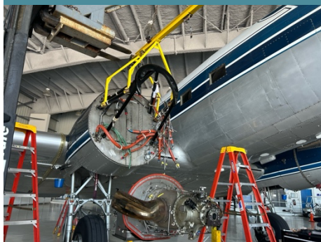
Removing the timed out engine on 200MF
